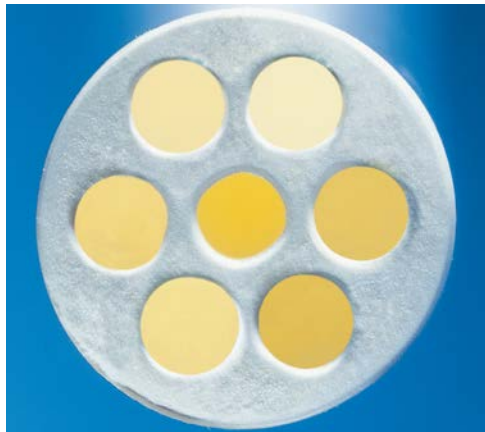
Figure 2-1: Multibore ® membrane developed by inge GmbH
