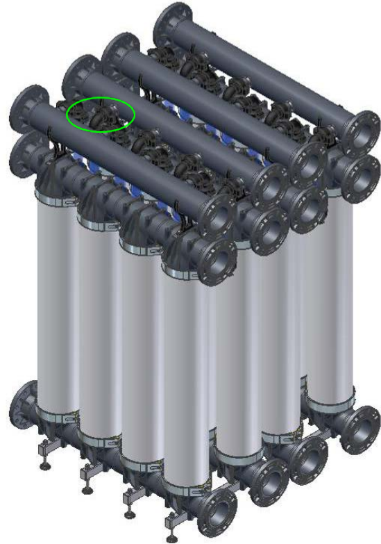
Figure 10-18: 2" couplings on filtrate header, four-row
