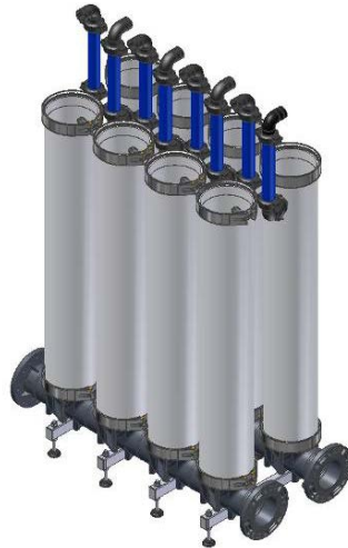
Figure 10-12: Assembly of top pipe coupling
