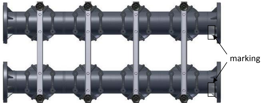
Figure 10-5: Bottom feed/drain header
