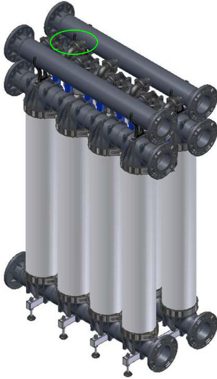
Figure 10-17: 2" couplings on filtrate header, two-row
