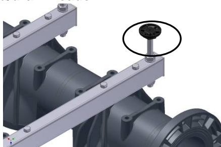
Figure 10-6: Attaching the adjustable feet
