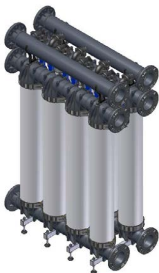
Figure 10-15: Installing the filtrate header
